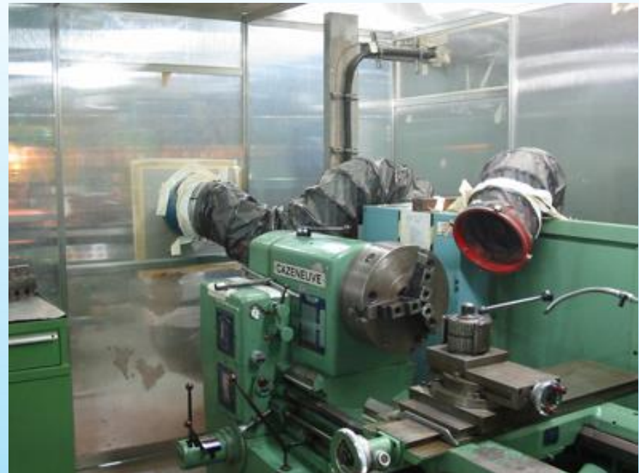
Inside the work site : aspiration
